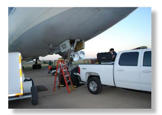
On-site installation of strain gages on the nose gear drag length of a Boeing 747. The drag length was instrumented as a full bridge transducer to measure towing force aplied to the landing gear during towing. Calibration was performed using a Tovey fatigue rated 100 klbf load cell installed in a modified tow bar.
